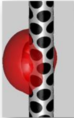
Figure 1. The design of the 64 contact DBS electrode (Sapiens Steering Brain Stimulation B.V., Eindhoven, The Netherlands).
